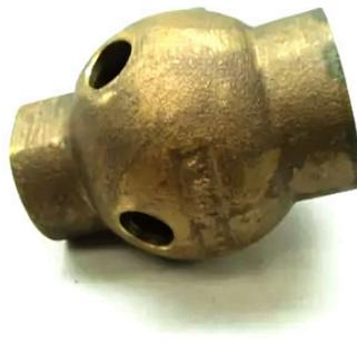
Penberthy NWH bronze steam jet heaters are available for freeze protection (installation by others) in cooling tower cold water basins. Live steam, as required, is injected directly into the water when used in conjunction with the steam basin heater controller and a steam valve with related piping.
