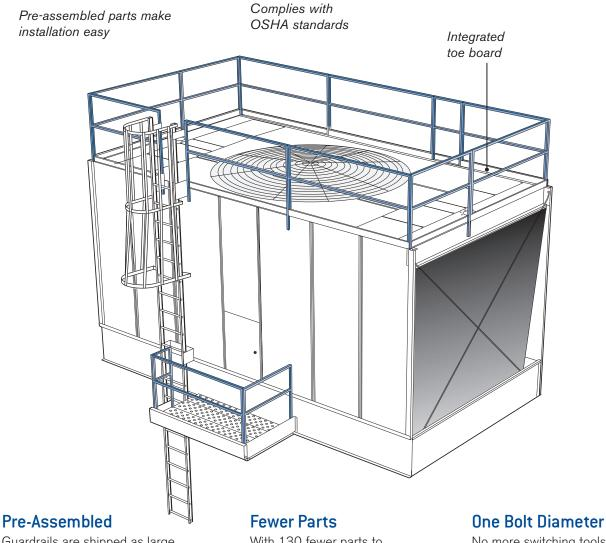
Guardrails are shipped as large welded sections that are self fixturing for easy and simple installation.
