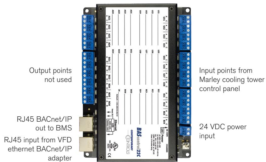
**Note:** CoolBoost fluid cooler control panels require two I/O modules
